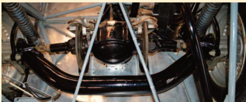
It is a non-independent beam or tube rear suspension system. Also known as a “dead axle” because it doesn’t transmit power to the drive wheels. It holds the rear wheels parallel and is not connected to the chassis. Thus, it reduces unsprung weight. It was used on race cars in the 1950’s and 60’s. Including Ferrari, Lotus, Maserati and Alfa Romeo.
